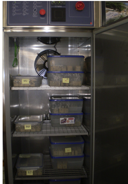
Fig. 2. EMC test sample boxes inside climate chamber.
